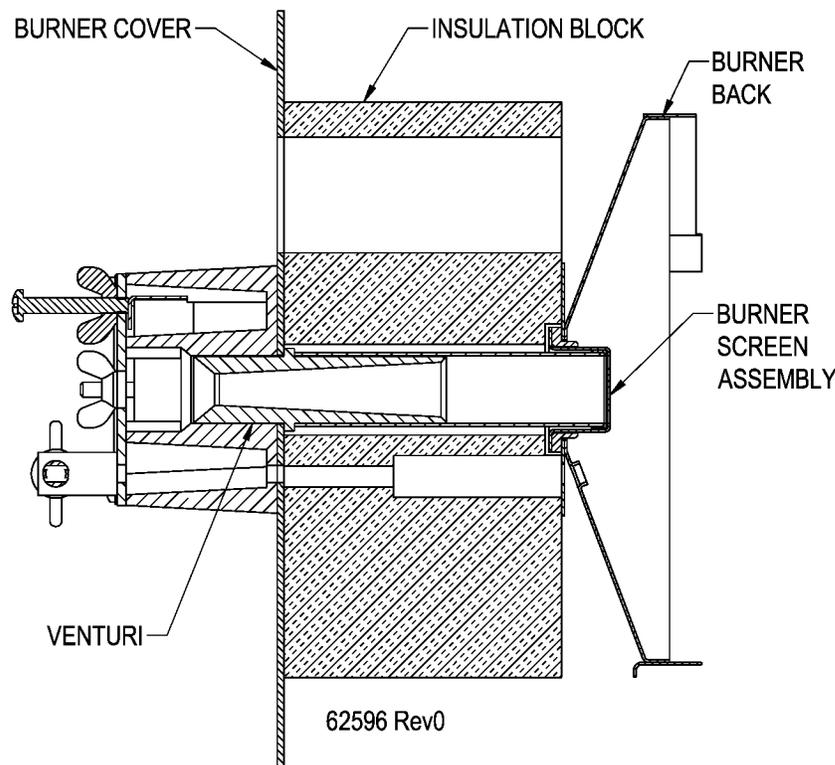
Figure 25 - Burner Assembly Cross Section
