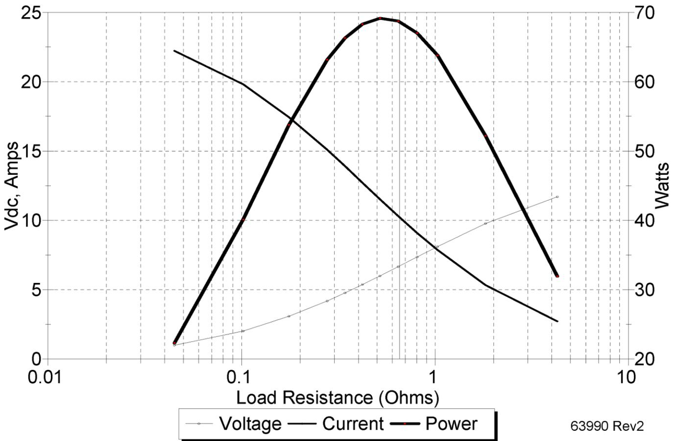
Figure 5 - Model P-5050 Power Unit Electrical Output Characteristics
