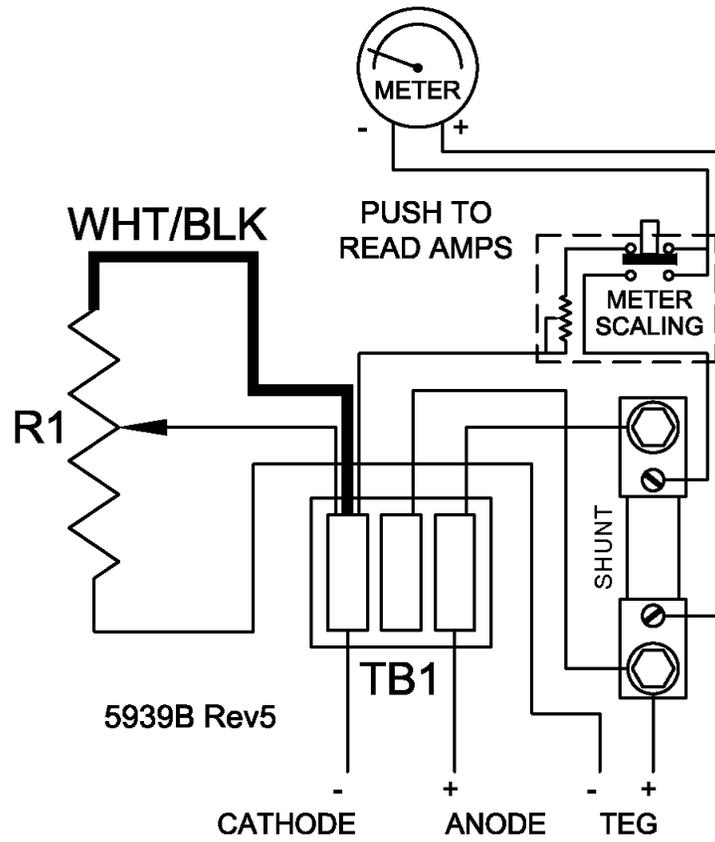
Figure 22 - CP Interface System, Series Wiring Diagram
