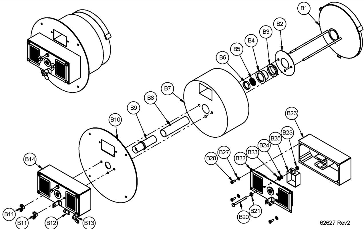
Figure 30 - Model P-5050 Burner
