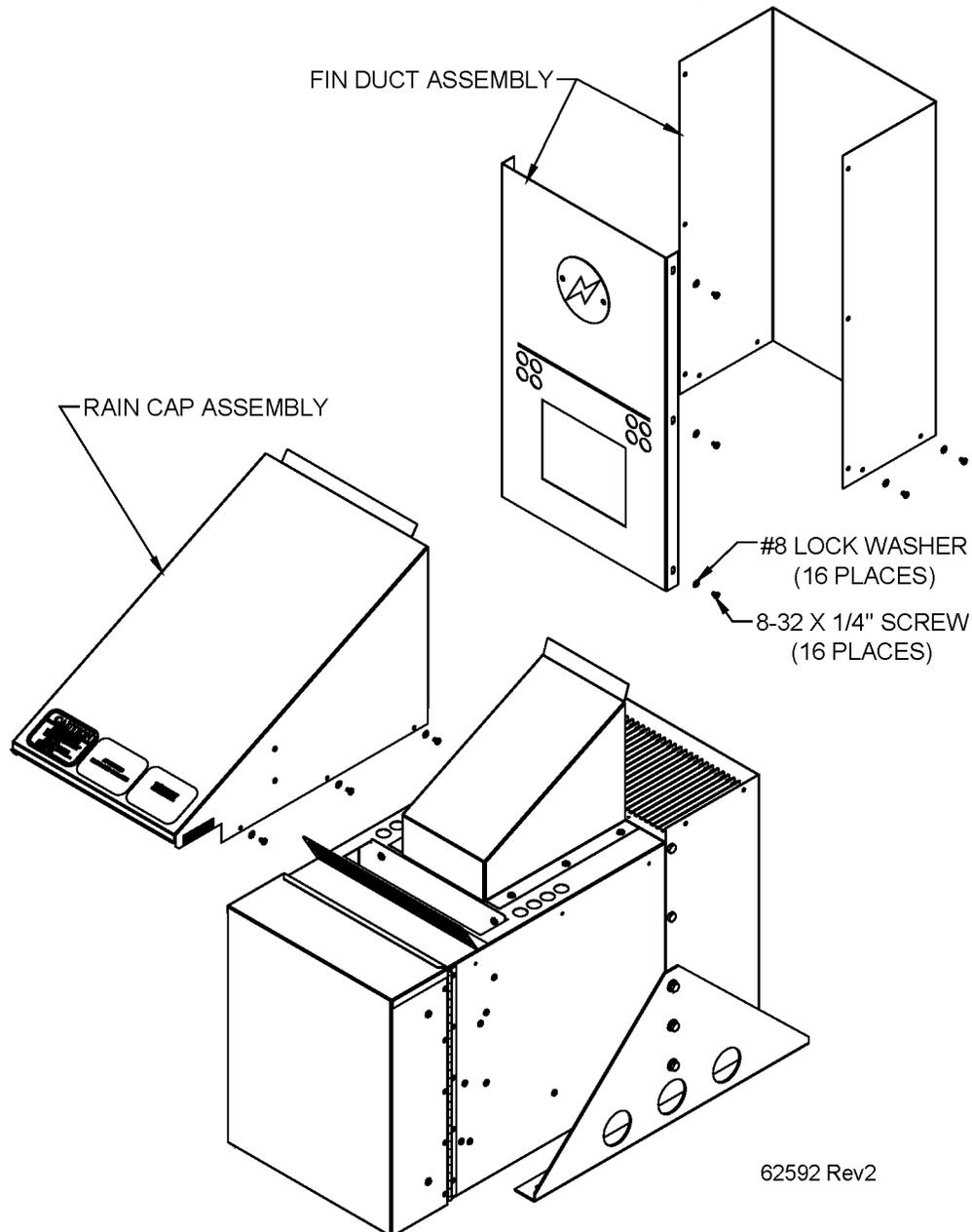
Figure 9 - Assembling the P-5050 TEG
