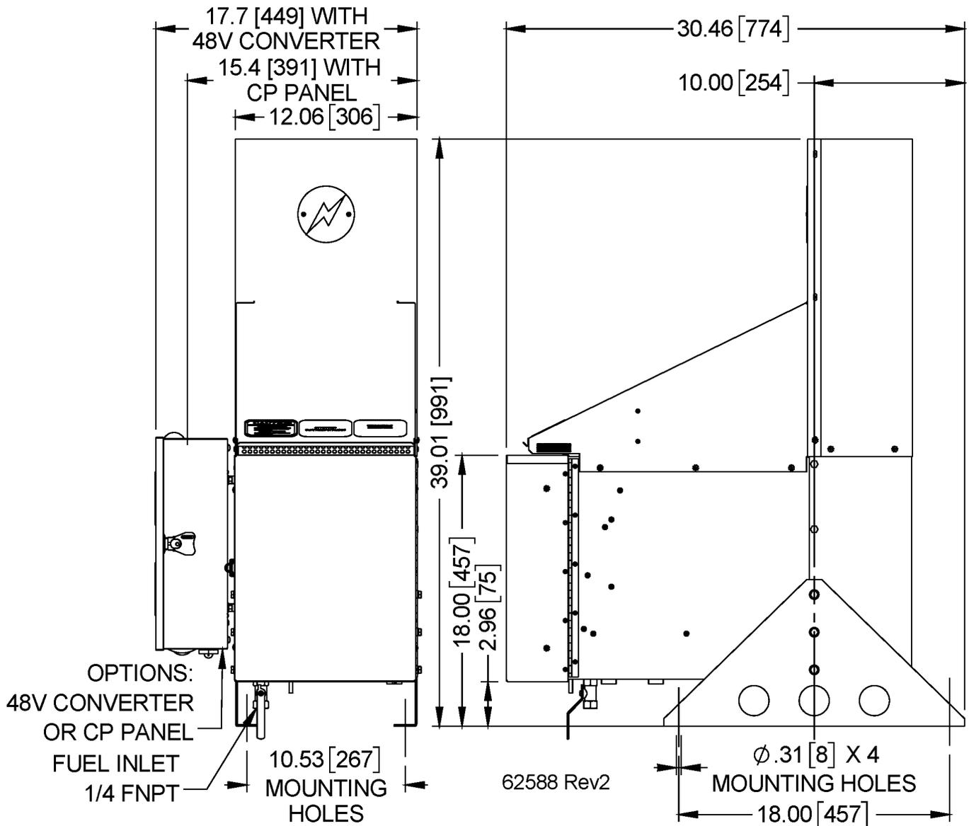
Figure 10 – Model P-5050 Mounting Dimensions
