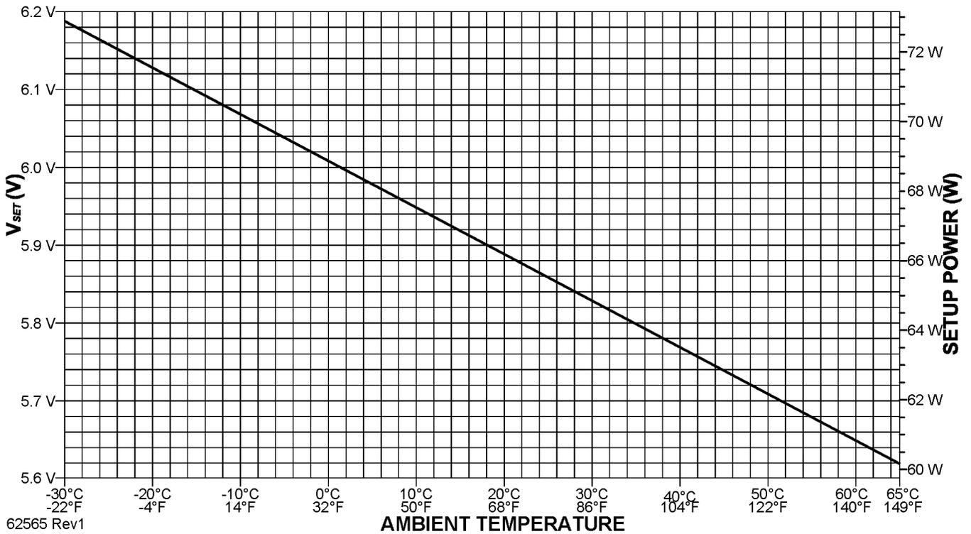
Figure 17 - V<sub>SET</sub> and Setup Power Versus Ambient Temperature
