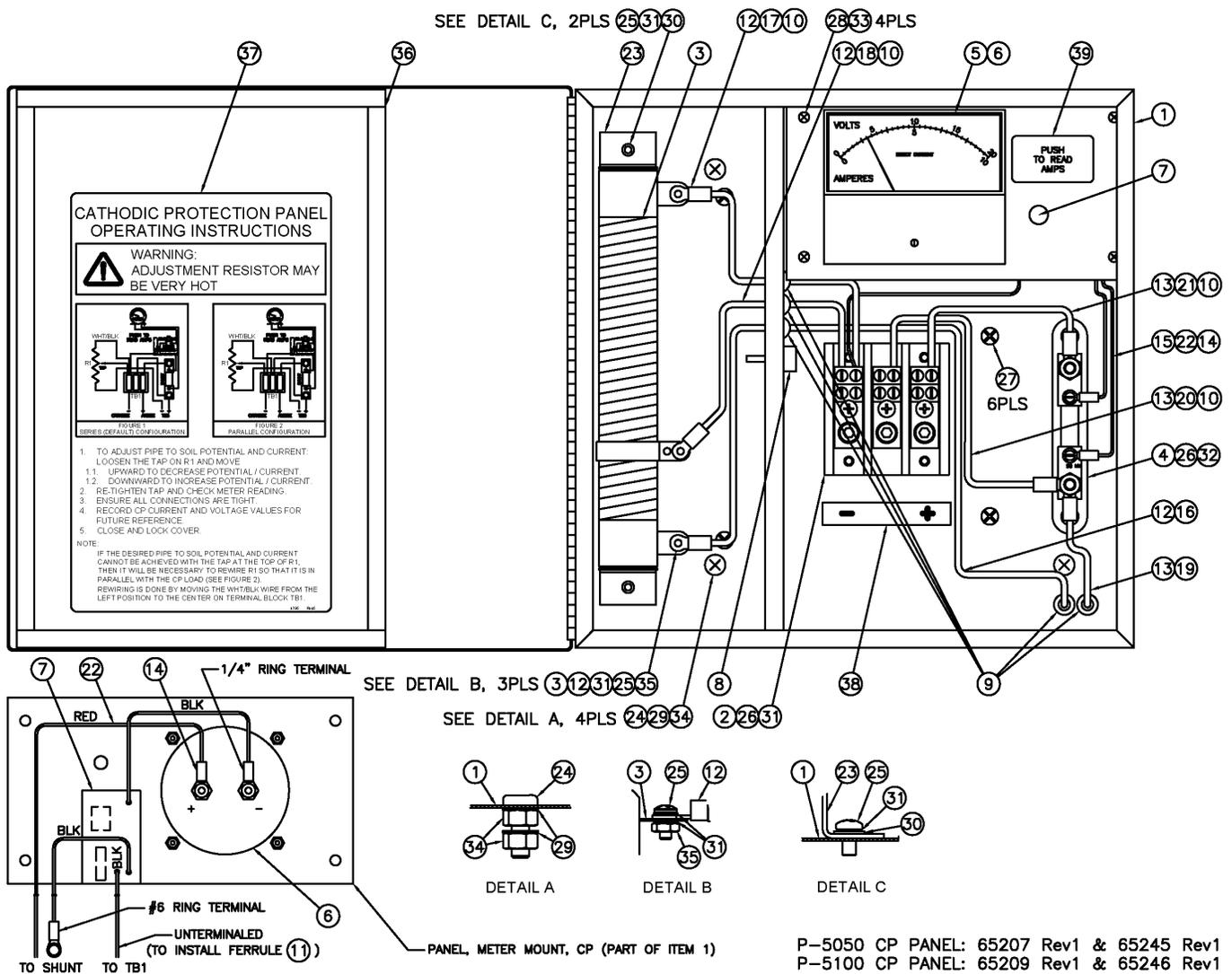
Figure 35 - Cathodic Protection System Parts Identification
