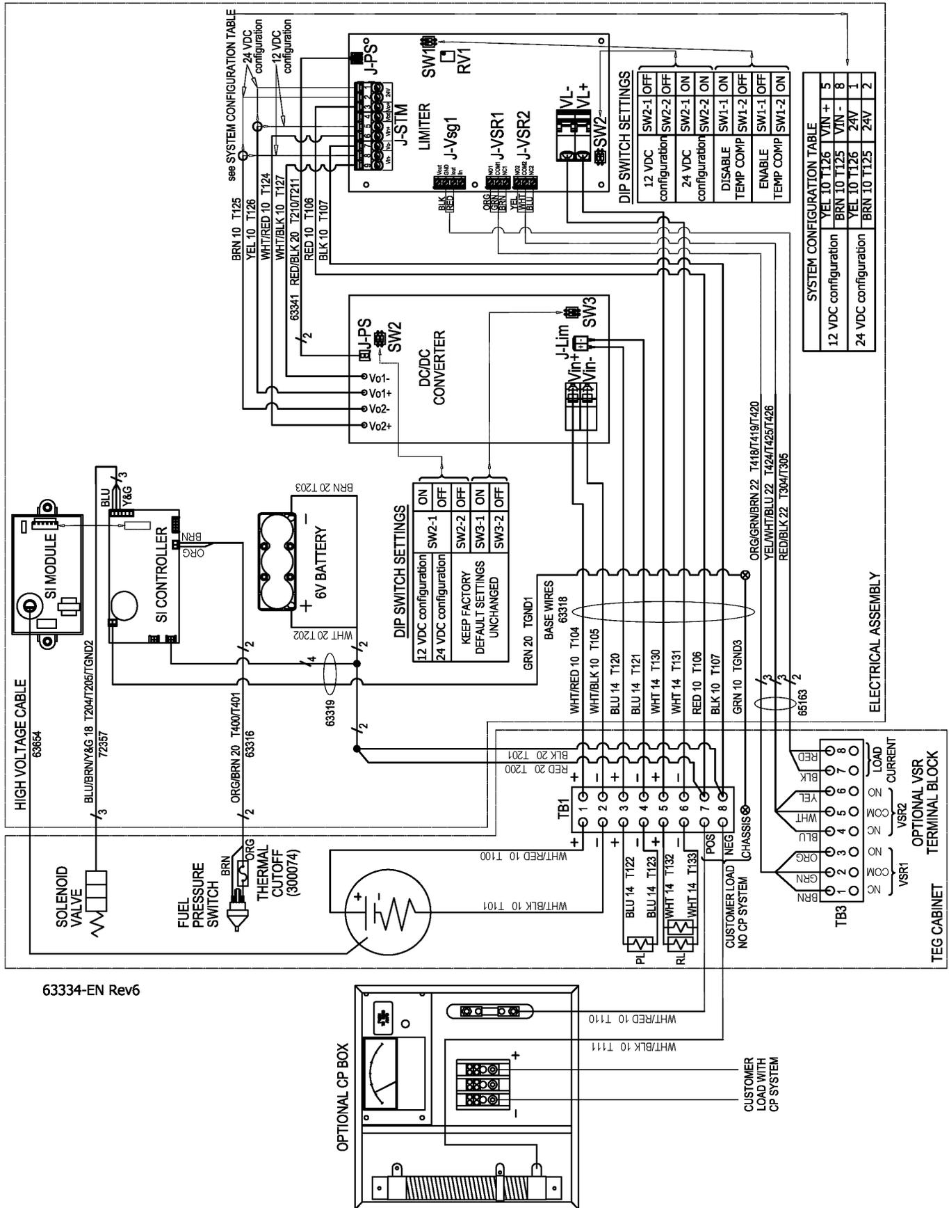
Figure 13 - Wiring Diagram P-5050 for 12 or 24 V
