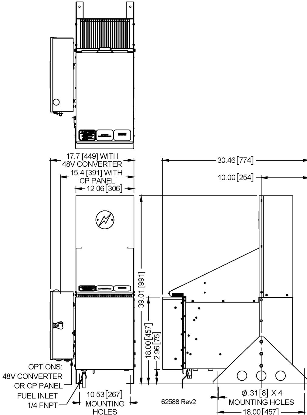
Figure 1 - Overall Dimensions of the P-5050 TEG
