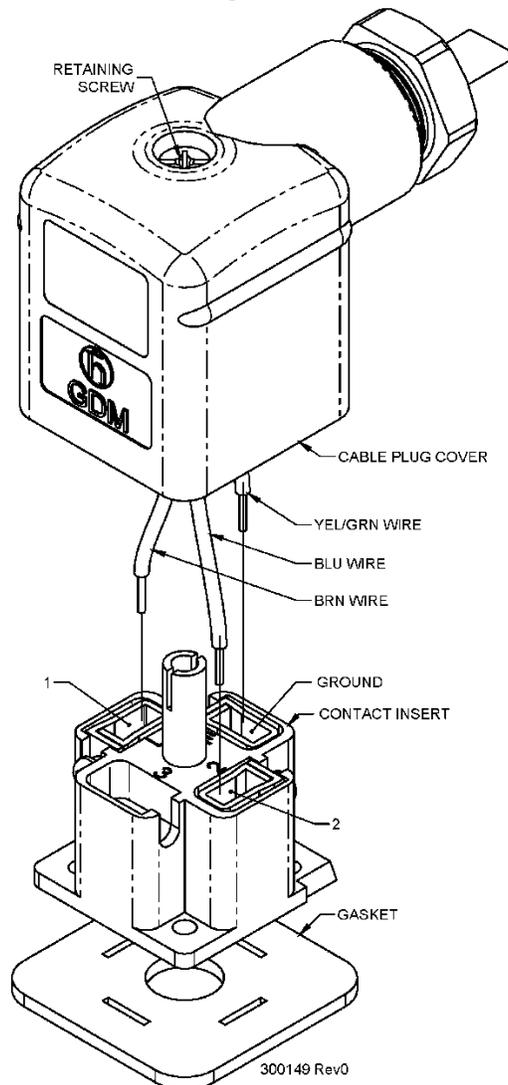
Figure 27 - Solenoid Valve Cable Plug Connections
