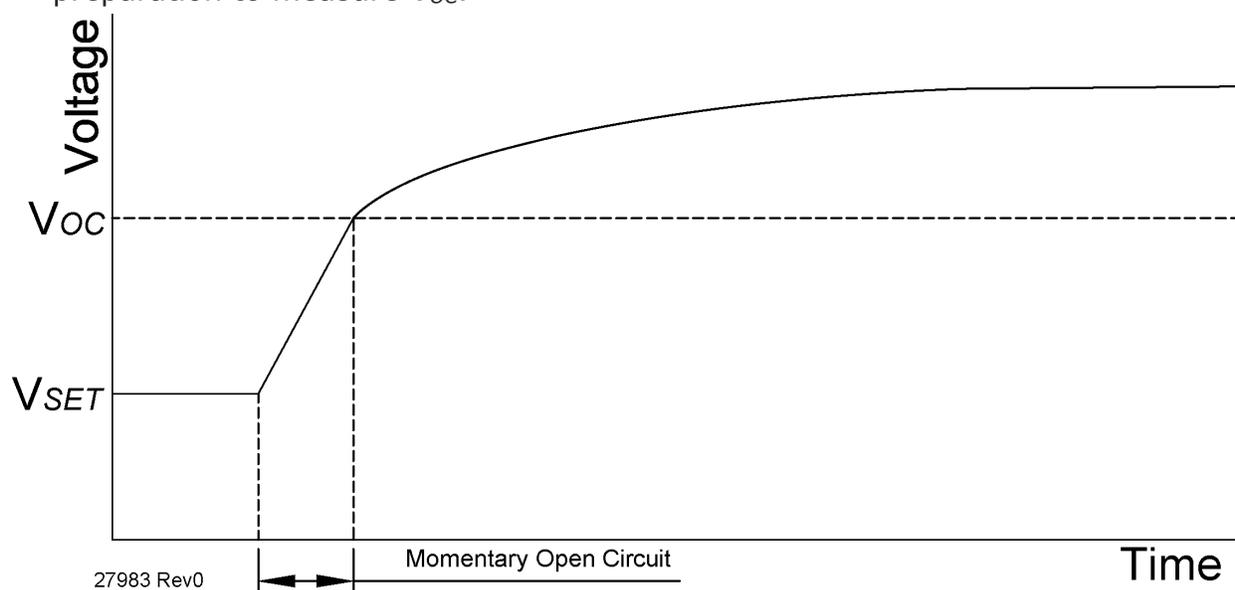
Figure 28 - Momentary Open Circuit Diagram
