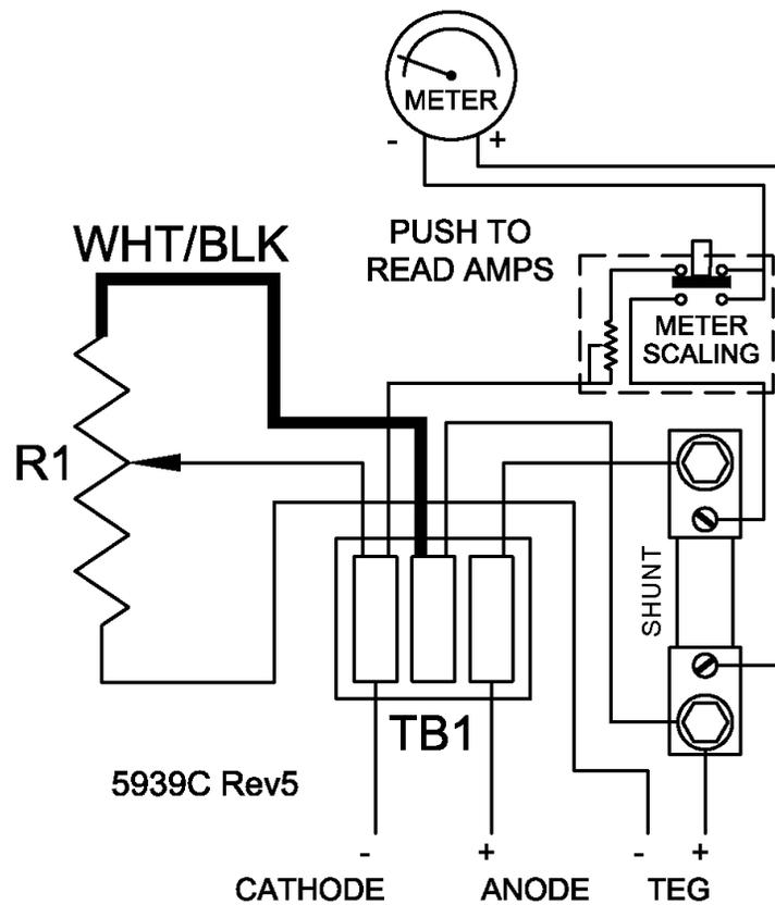
Figure 23 - CP Interface System, Parallel Wiring Diagram
