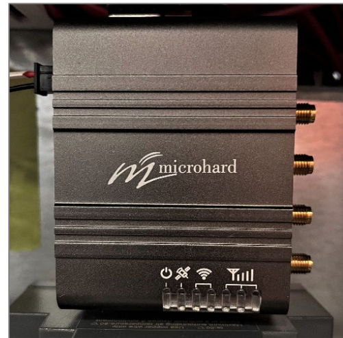
Figure 8-1 – Cellular Modem Located in the Electrical Enclosure
