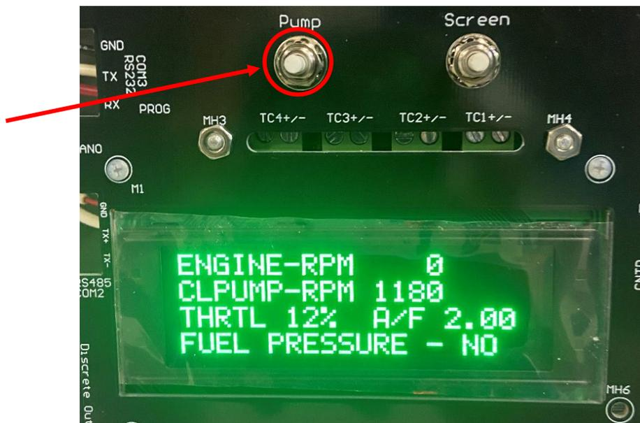
Figure 11-4 – Pump Button Location
