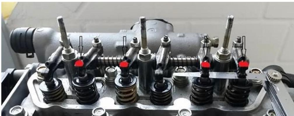
Figure 14-2 – Rocker Arm & Valve Stem
