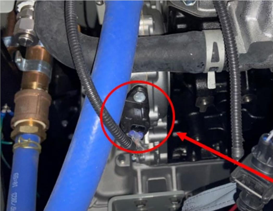
Figure 12-11 – #7 Crank Position Sensor
