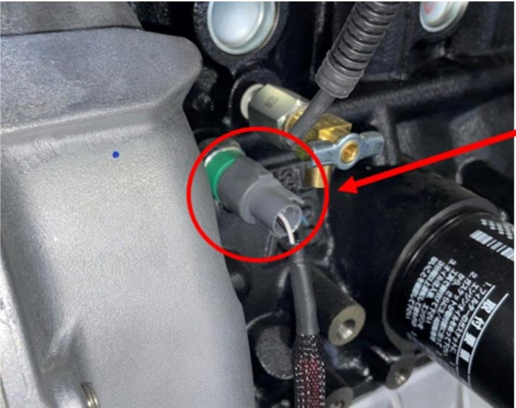
Figure 12-10 – #6 Oil Pressure Sensor / Switch
