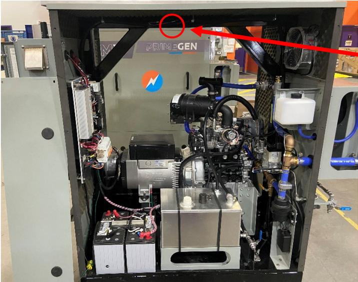
Figure 12-17 – Thermal Fuse (Engine Room)
