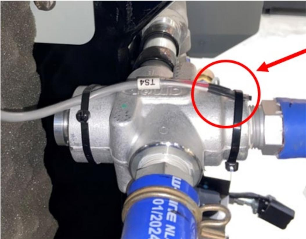
Figure 12-6 – #2 Radiator Outlet Temperature Sensor
