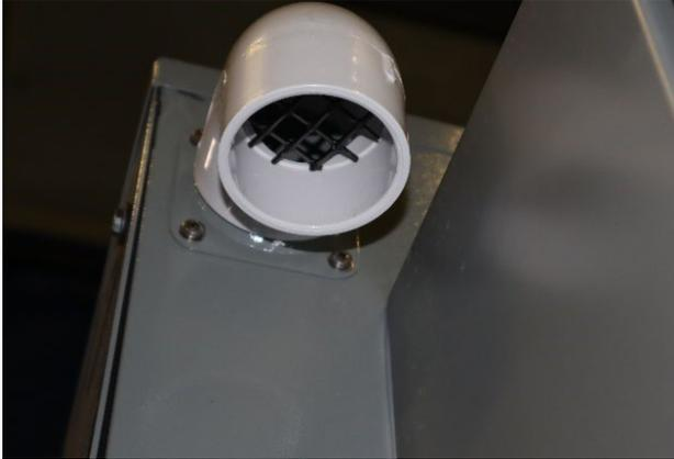
Figure 8-1 – Engine Air Intake
