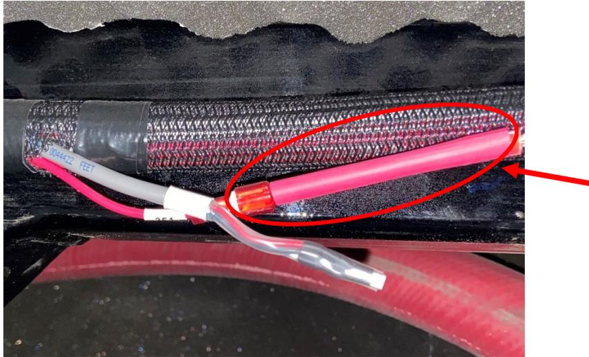
*Figure 12-18 – Thermal Fuse (Engine Room)*
