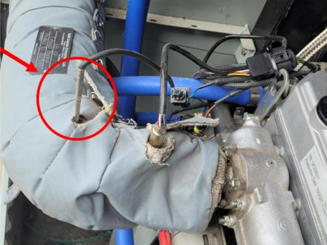
Figure 12-12 – #8 Exhaust Temperature Sensor
