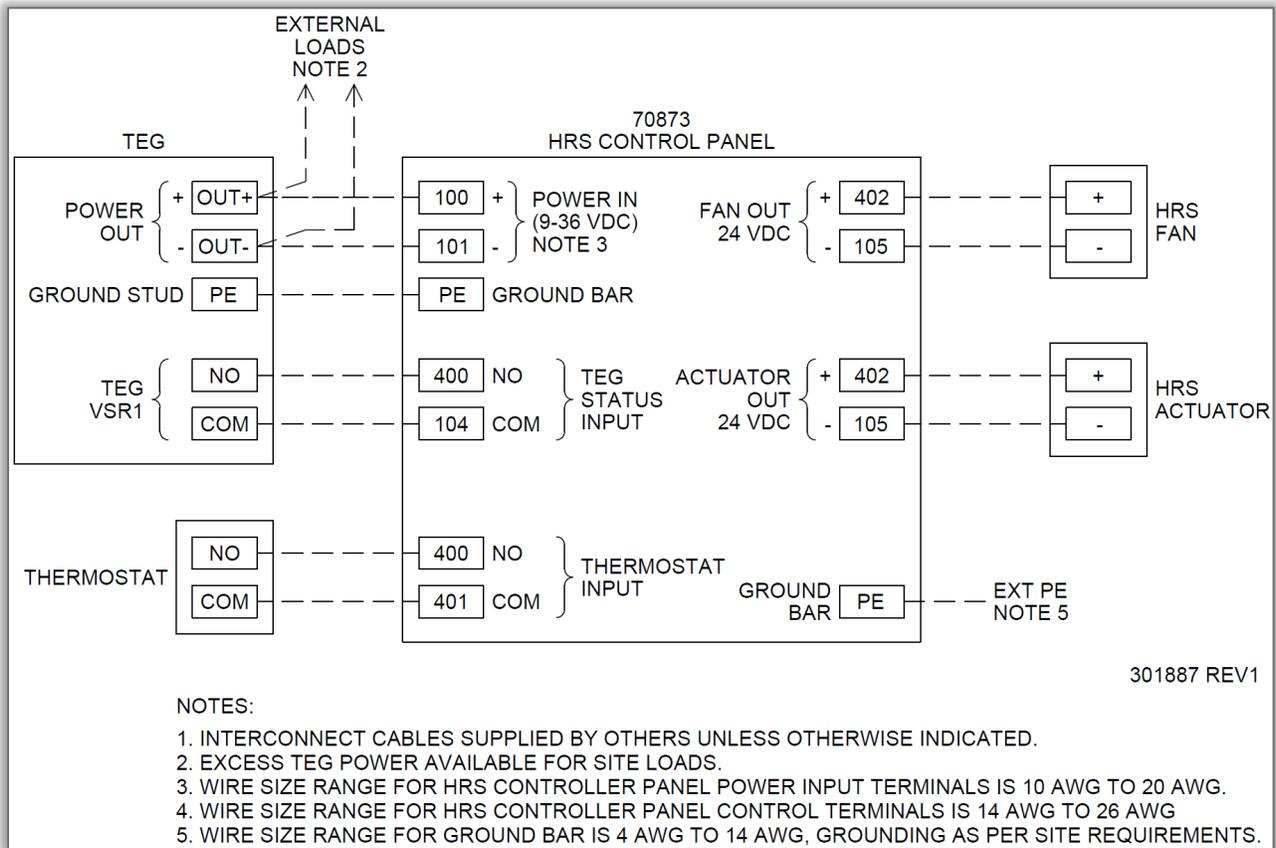
Figure 5 – Wiring Diagram for Heat Recovery Systems
